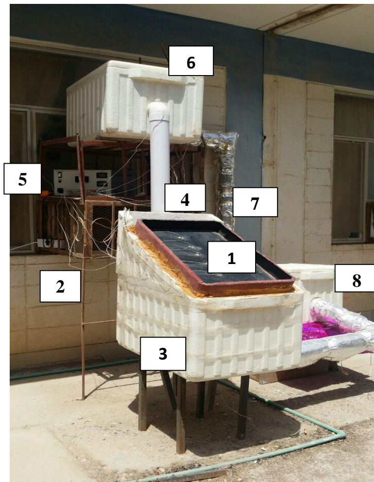
1-Storage plate. 2-Thermocouple "K".3-sollar collector.4-pipe . 5-H112 .Heat transfer service unite (HTSU). 6-Paraffin room . 7-Insulation. 8-Cooling room.
